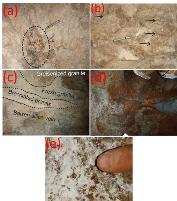
Fig. 4 Field photographs show the alteration features of El-Missikat pink granite through DI and DII: a brecciation, b silicification, c greisenization, d hematitization, and e kaolinization
