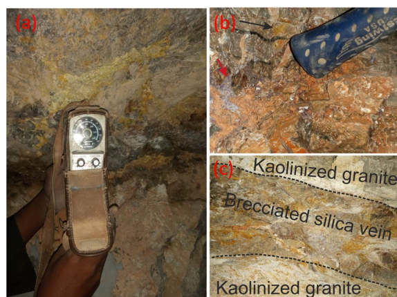
Fig. 6 Field photographs show the occurrence of yellowish-greenish yellow secondary U minerals, at DI of El-Missikat shear zone, as fracture infill hosted by the brecciated silica veins a and associated with fluorite ( b -look at red arrow), with occasional occurrence through the kaolinized granite ( c )
