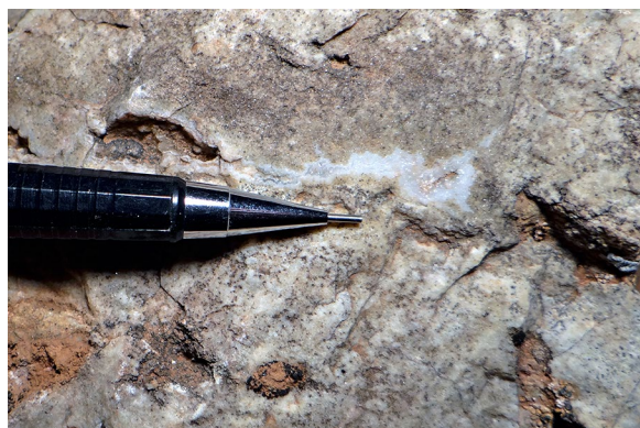
Fig. 3 Example of translucent to white secondary silica from the Kaibab Formation chert rubble breccia (Sevenmile Draw). Vugs are typically rimmed with fibrous silica which transition to drusy quartz toward the middle of vugs, interstices or cavities. Mechanical pencil tip (width) is 0.05 mm
