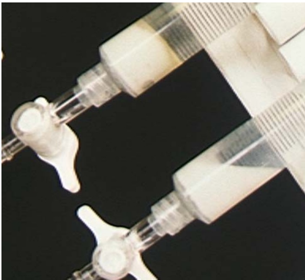
Fig. 2 Bioreactors containing glass beads ( 100 \mu\text{m} ). Upper bioreactor was inoculated with A. coffeaeformis 10 d previously. At this time diatoms were no longer growing and matrix polymer formation was well developed. Lower bioreactor is uninoculated control. Note avalanching of beads in the uninoculated control.
