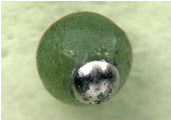
Figure 14 Photography of the reduced herzolite-metal oxide mixture. Metal exsolved from the silicate. The diameter of the sphere was ~2 mm. The material was levitated with a mixture of 98 vol.% Ar and 2 vol.% H 2 .
